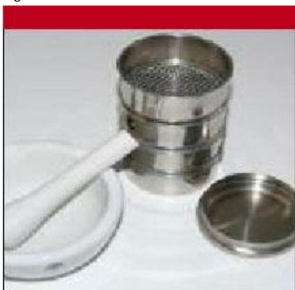
**Figure 4:** Mortar and pestle and sieve set.
