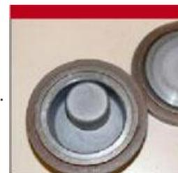
Figure 5: Tungsten carbide grinding container.
