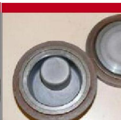
**Figure 5:** Tungsten carbide grinding container.
